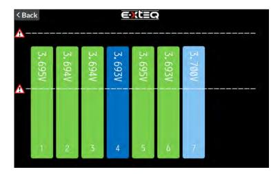
The cell with the lowest value is in blue. The cell with the highest value is in sky blue.
