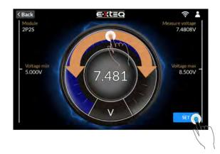
Click the center of the gauge where the value is displayed, a keypad will display to input the exact value. Confirm the value by taping "Ok".
