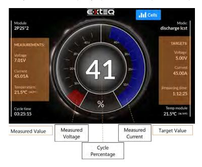
To see the cells charging in detail, tap on 'CELLS" tab.
