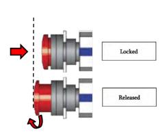
Make sure "Emergency switch" is released before powering on the machine. (Turning clockwise will release the switch).
